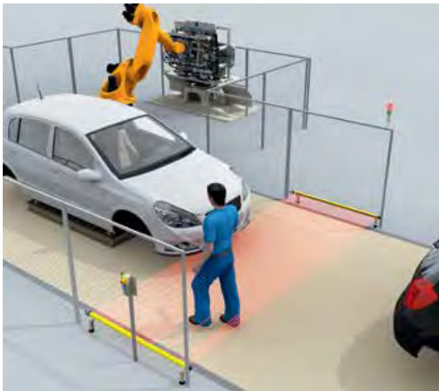
Entry/exit function with horizontally installed safety light curtain in a processing station on an automobile assembly line.
