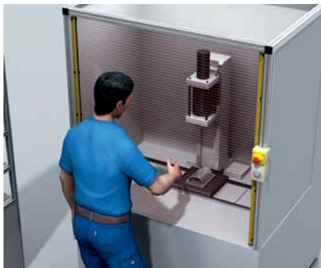
Hazardous point protection using a safety light curtain
